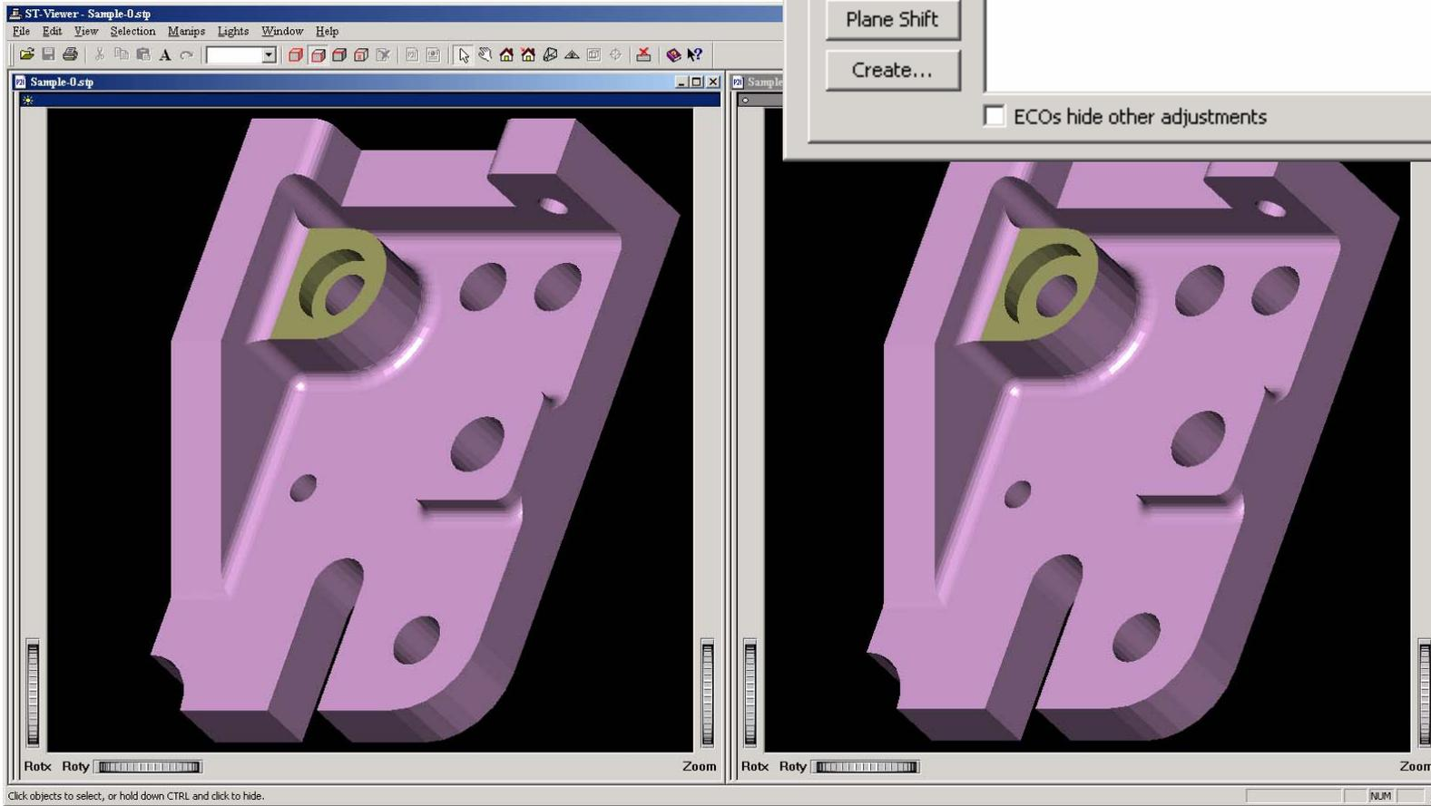
The only surface modified exclusively by [Raise Boss] is the fillet shown in gold. The adjoining planar surface shaped like a “D” was the actual surface that was moved in the CAD system, but one of it’s edges was also modified by the change in the counterbore diameter.
