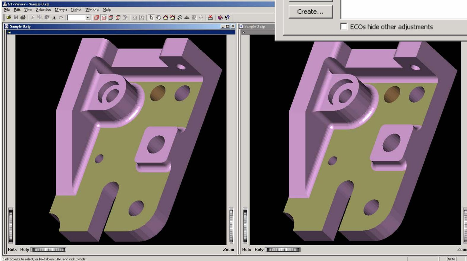
Adjustment [Incr Clearance 1] is another radius change, but not as simple. Observe that all the surfaces are olive colored this time (no gold surfaces). This tells us that none of the surfaces was modified exclusively by the highlighted adjustment. The other change will be apparent later in the next step of this tour.
