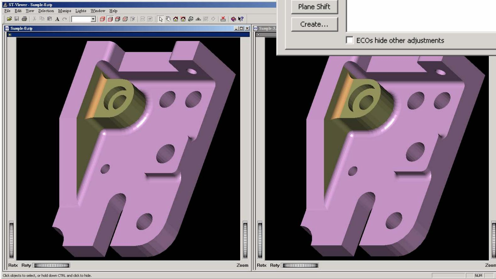
We highlight adjustment [Stretch] to show surfaces modified by stretching the part. The surfaces shown in purple were not part of the stretch, the surfaces shown in gold were stretched. The surfaces shown in olive had some edges modified.
