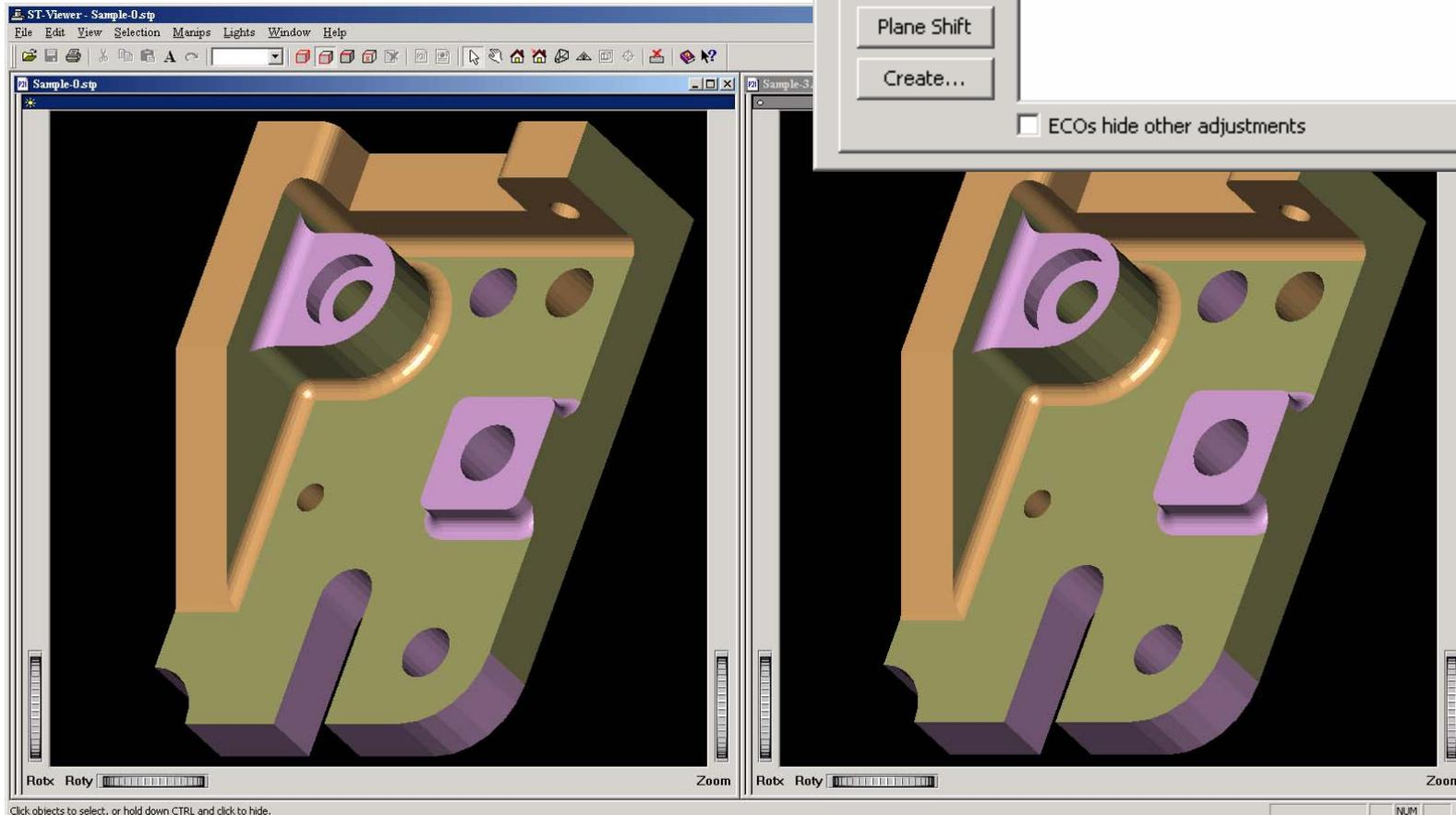
When the user selects adjustment [Incr Clearance 2] to highlight the change of a radius (one place in this case) from 0.22 to 0.23. The adjustments can be renamed to more meaningful names by the user.
